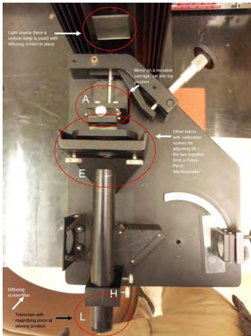
Figure 9: The Fabry-Perot interferometer setup used in this experiment — letters indicate units, as noted in the explanation above.
