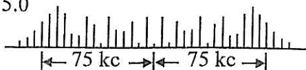
Frequency spectra of frequency-modulated waves, showing effect of varying the frequency deviation, for constant modulating frequency.
