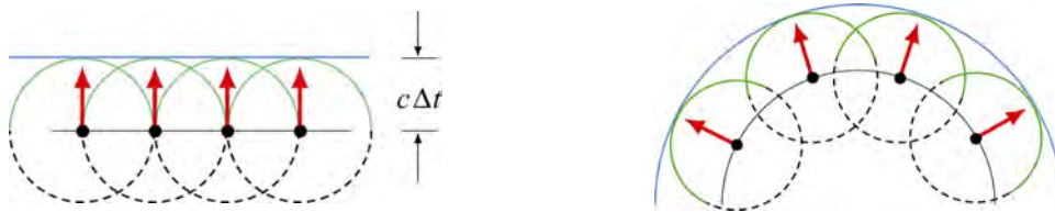
Figure 14.4.1 Propagation of wave based on Huygens's principle.
