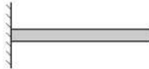
Figure 33: Uniform cylindrical rod fixed at left end.
